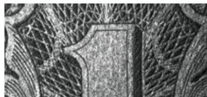
UV Lens with near UV light. The texture of material and unevenness of ink can be recognized
