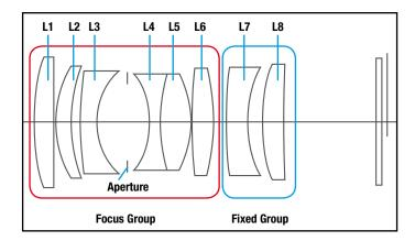
A floating focusing mechanism focuses whilst changing the spacing of some of its optical systems in order to minimize changes in aberrations due to object distance. The lens's construction is divided into a focus group that moves when focusing and a fixed group that remains stationary.
