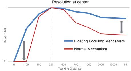
MTF is significantly increased at not only shorter working distances for machine vision applications but also at distance for intelligent transportation systems, making the lenses suitable for use at all working distances.
